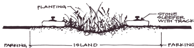
Sketch B. Sleepers and tracks used to delineate parking islands/rain gardens from parking.
